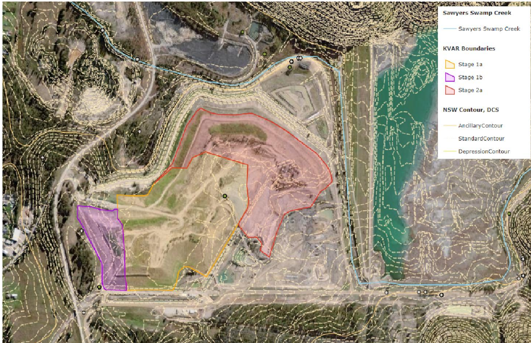
Figure 1.2 Historical ash placement at the cessation of ash placement KVAR Stages 1 and 2
